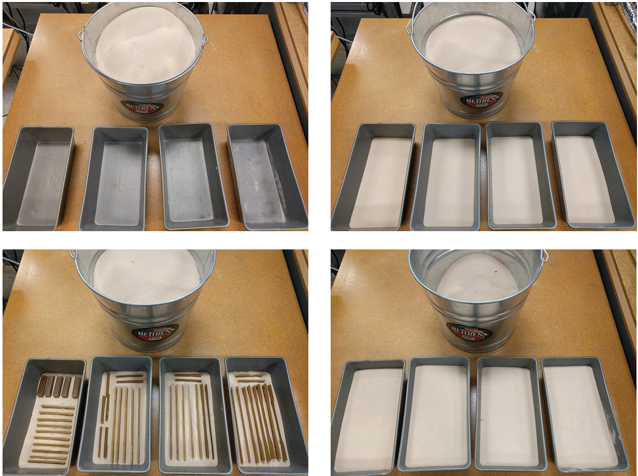
Figure 2: Specimens should be placed in a sand bath to prevent deformation while being annealed.
