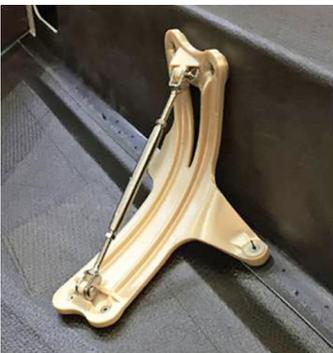
Manufacturing tool 3D printed using ULTEM™ 9085 resin enables Indaero to produce complex shapes that perfectly fit the curvature of aircraft panels not possible with traditional aluminum tools.
