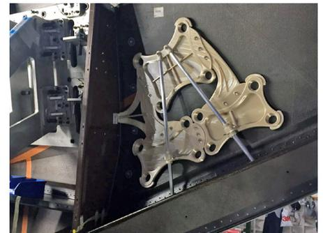
New 3D printed manufacturing tool produced using tough ULTEM 9085 resin material fits against a curved panel independently, freeing up operators and accelerating customer delivery times.
