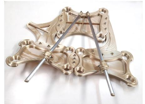
Indaero redesigned and 3D printed a tool nine kilos lighter than the traditionally manufactured tool.
