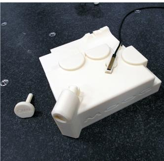
With Stratasys 3D printing technology, Moog Aircraft Group produces CMM fixtures in a matter of hours rather than weeks.
