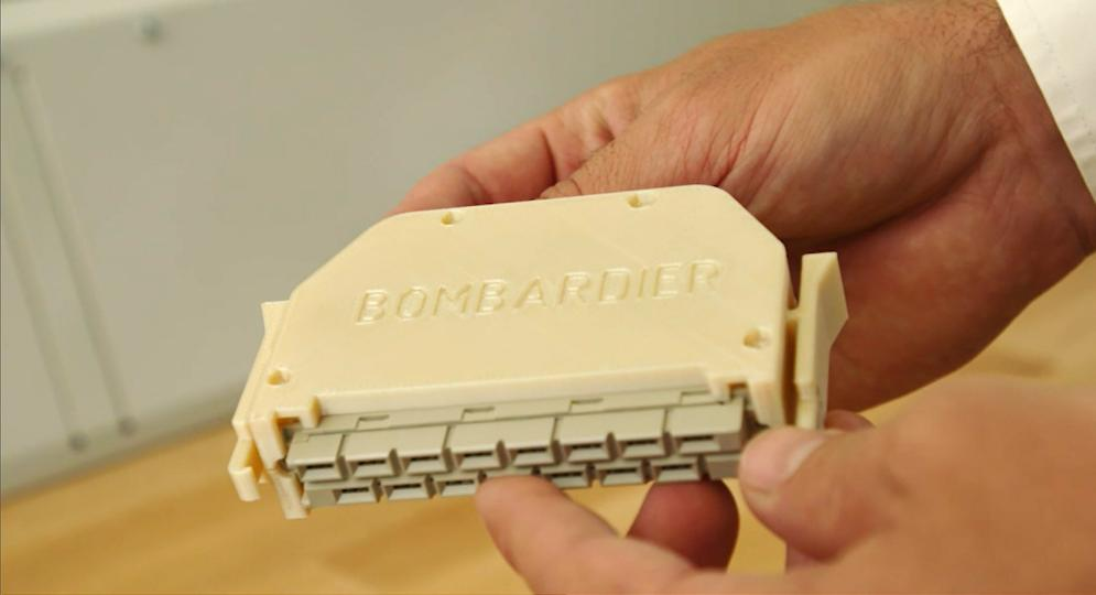
3D printing train parts like this connector with the F900 saves nearly 77 percent in production time.
