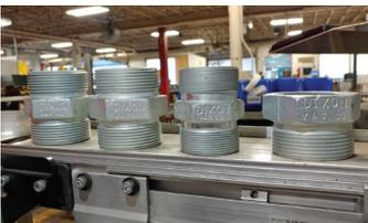
Dixon gaskets are inserted into these fittings using a SCARA robot and 3D printed grippers.
