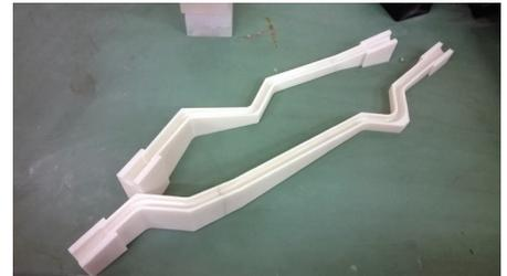
Solidify leverages 3D printing to make tools and jigs to manufacture parts for the automotive industry.
