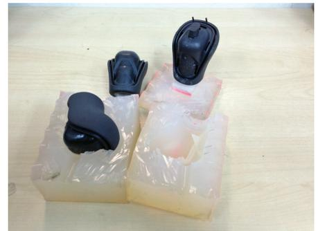
Solidify 3D printed a master part to create these silicon rubber molds for their automotive client.
