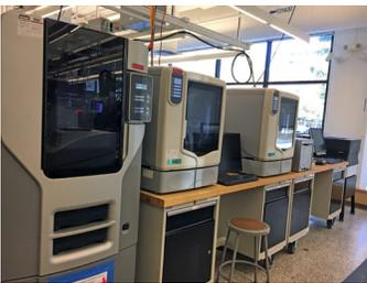
Some of the Stratasys FDM 3D printers at the Engineering Product Innovation Center (EPIC) at Boston University. The center also has PolyJet 3D printers, including a Connex3™.
