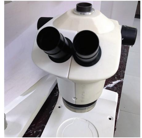
The 3D printed binocular body cover painted white on the left side
